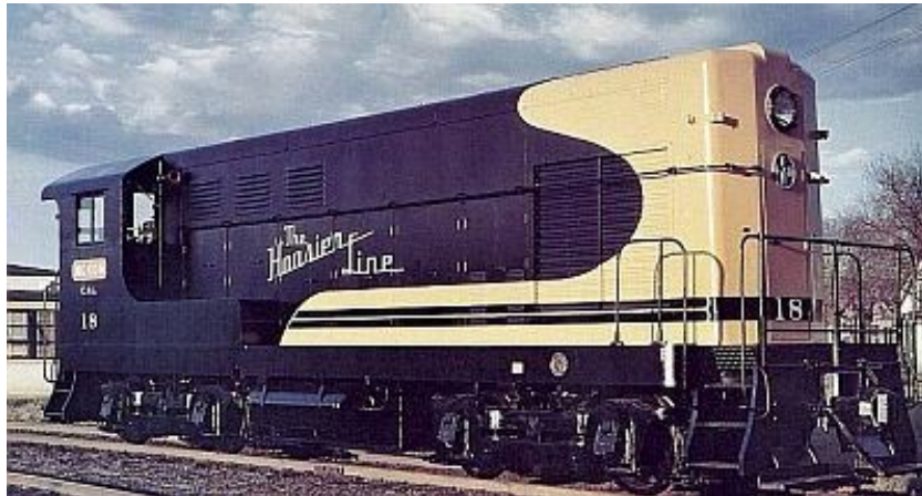
H-10-44/ 1000 HP B-B switcher
