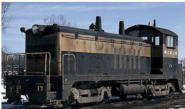
NW-2 / 1000 HP B-B Switcher
