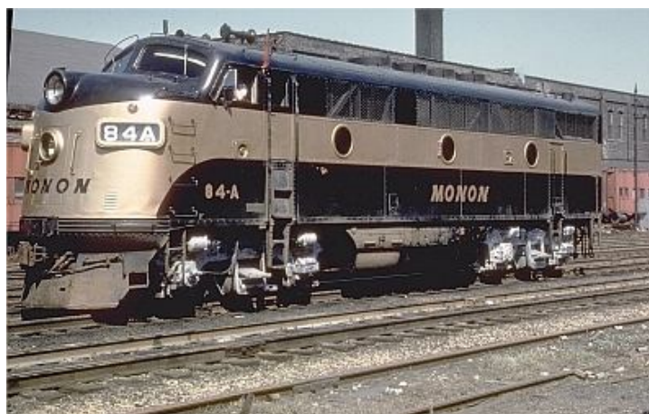
F-3 1500 HP B-B Streamlined Cab Unit Original Freight Units
