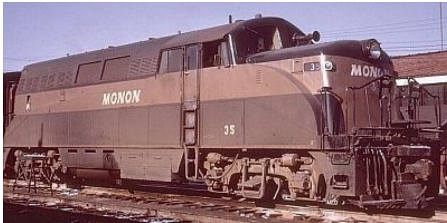
BL-2/ 1500 HP B-B, semi-streamlined road switcher
